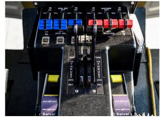
As with most aircraft, there is an array of controls that are truly baffling if you don't know them, but spend a little time looking over them and it becomes much clearer. Fire-suppression systems, circuit breakers and fuses adorn the roof, along with big levers to let our air from the ballonets and helium from the envelope – although that's an undesirable thing to do. There's also a huge amount of redundancy common to all aircraft – 'if this fails, we have that' and so on.
