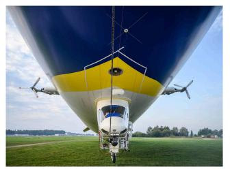
Although this Zeppelin could be lighter than air, typically it isn't. Instead, it's ballasted to a weight of around 300-400kg. Like a shark, then, which sinks if it stops swimming, the Zeppelin has negative buoyancy. Helium accounts for 95-97% of its lift, with the rest, in cruising flight, coming from aerodynamics, either across the control surfaces or by pitching its nose upwards by anything from as little as 1deg to as much as 8 deg if it's heavily laden.
